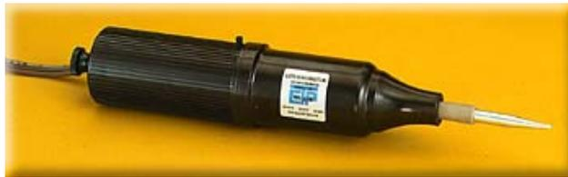
**DESCRIPTION.** The Model BD-10A and BD-10AS are hand-held units which generate a high voltage at a high frequency. **It is intended for intermittent use, no more than 10 minutes at a time.** It has an output of between 20,000 to 45,000 volts, at a frequency of approximately 500 kHz. When properly adjusted, when the electrode is held within  $\frac{1}{4}$  to 1 in. (6 to 25 mm) from a metal object, a spark will jump to the metal. Current output of the spark is about 1 mA.
