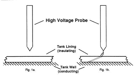
Figure 1. Spark testing a tank lining. No hole is present in (a), and no spark discharge occurs. A hole is present in (b), and a spark discharge can be seen between the probe tip and the point at which the hole intercepts the top surface. The oblique hole sketched in (b) is longer than the lining surface.
